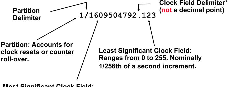
Most Significant Clock Field: Ranges from 0 to 4294967295 (2<sup>32</sup>-1). Nominally 1 second increment.
