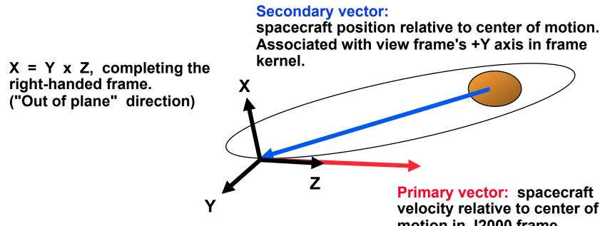
Normalized component of secondary vector orthogonal to primary vector. This vector is aligned with the view frame's +Y axis. ("In plane" direction) Primary vector: spacecraft velocity relative to center of motion in J2000 frame. Associated with view frame's +Z axis in frame kernel. ("Down track" direction)
