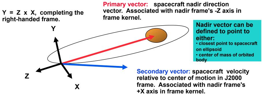
Normalized component of secondary vector orthogonal to primary vector. This vector is aligned with the nadir frame's +X axis.
