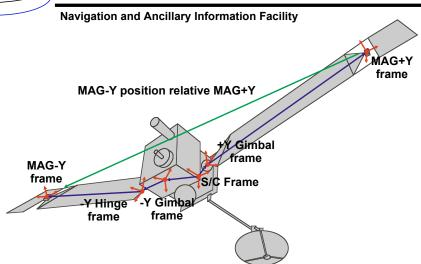
Find the position of one MGS MAG sensor with respect to the other in the MGS s/c frame. Also find the relative orientation of sensors:
